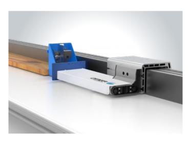
The pneumatic tail clamp (optional), assures a high precision length positioning with a tolerance of +/- 0.15 mm at a maximum feed speed of  $60\,\mathrm{m/min}$ .
