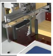
Detail of the cutting area with "Intelligent" front and vertical clamps, riding on high precision linear bearings. The see-through polycarbonate guard allows for a clear line of sight to the area of the operation of the saw and easy access to the compartment for maintenance, through the assisted lifting of the guard.
