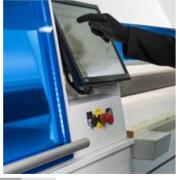
CNC, with Windows Embedded OS and connected to an adjustable 17" Touch Screen display, allows the easy and comfortable use to any operator, reducing vision fatigue and ensures a natural touch on the screen
