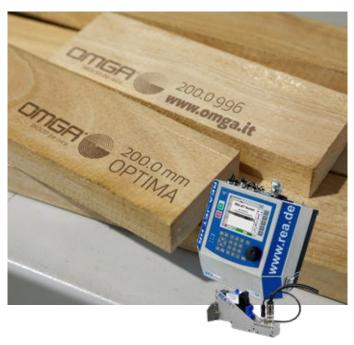
$\label{thm:light} High \, resolution \, INK-JET \, printer \, for \, printing \, custom \, strings \, and \, logos \, on \, cut \, pieces. \, The \, system \, uses \, HP \, \big( Hewlett \, Packard \big) \, cartridges, \, which \, make \, it \, reliable \, and \, easy \, to \, maintain.$
