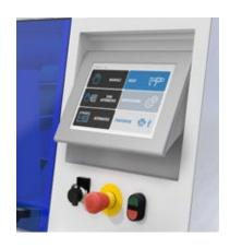
The numerical control, associated with the 10.4" industrial Touch Screen, offers the operator an easy data entry and an intuitive guide to the use of the various optimization programs. The adjustable Touch Screen display, allows the easy and comfortable use to any operator, reducing vision fatigue and ensures a natural touch on the screen.
