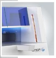
Safety barrier: allows the operator to work with maximum safety as, if interrupted, it immediately blocks the movement of the feeding carriage. The barrier is deactivated automatically when the carriage is working inside the machine cabinet, thus allowing the preloading of a new bar.
