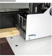
A vertical tail clamp fitted on the pusher, allows for feeding speeds of 240 m/min. while ensuring very precise length tolerance of +/- 0.15 mm.
